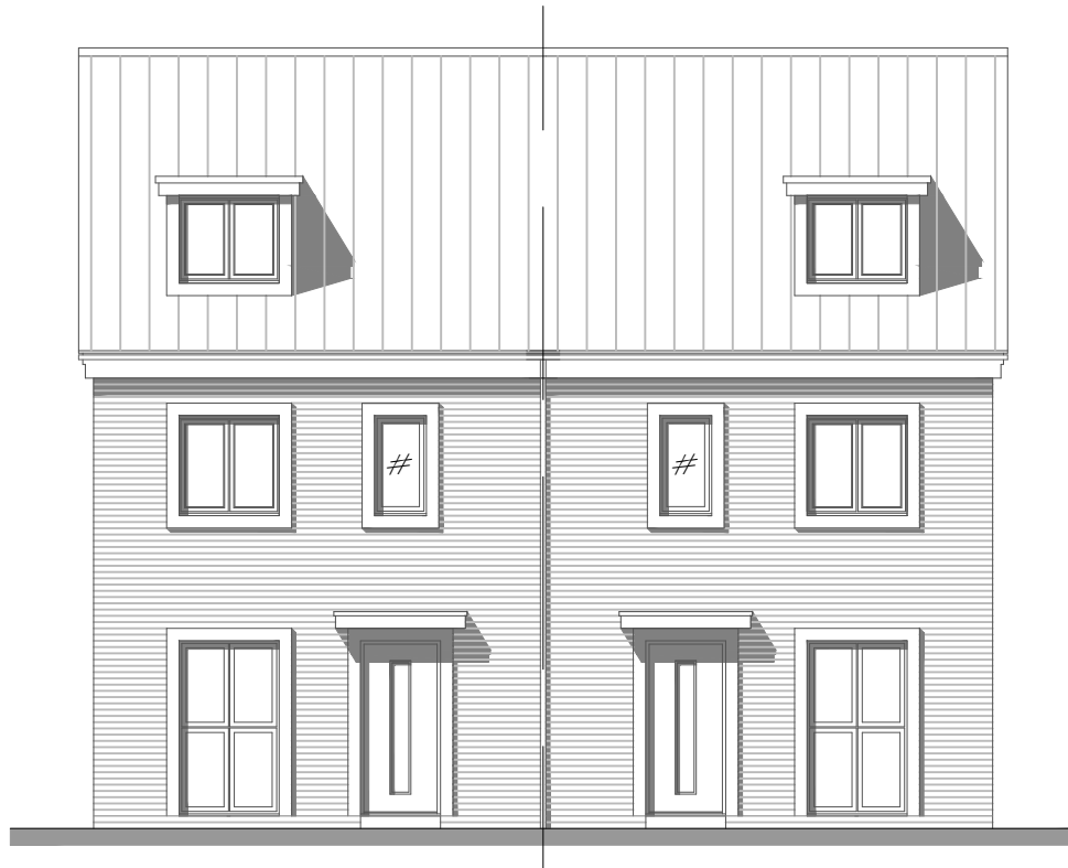
FRONT ELEVATION #-Obscure Glazing
